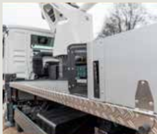
Jack boxes and turret tube made of high-strength fine-grained steel
